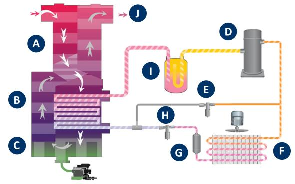
hot, moist compressed air enters the separate air to air heat exchanger where it is precooled
